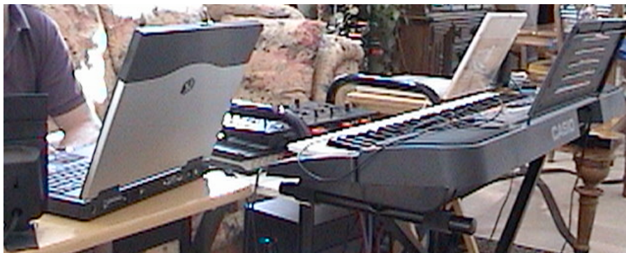
Figure 1.1 Unidentified Wailing Mammals recording setup including PC Laptop, Mixer, Apple iBook, MIDI Keyboard, Roland Sound module, and speaker setup.
