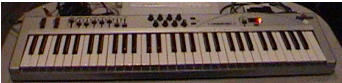
Figure 3.3 Basic Midi Keyboard Controller with 61 Keys, 9 Knobs, 9 Sliders, Pitch bend, and Modulation control.
